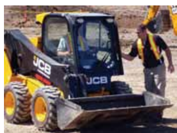
JCB Product Specialist, David Pendleton shows a potential customer the skid steer side entry door
